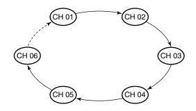
Normal scan, like priority scan, searches through all tag channels in sequence. However, unlike priority scan, Channel 16 is not checked unless Channel 16 is set as a tag channel.
